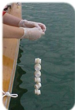
The integrative passive samplers (IPS) enable to monitor the chemical quality of aquatic medium. The technique of the diffusive gradient in thin film (DGT) is used for the determination of metals.
